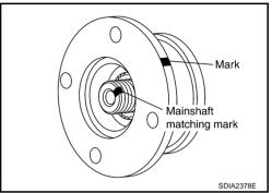
22. Tighten self-lock nut to the specified torque, with flange wrench. Refer to <a href="https://doi.org/10.1007/j.com/PONENTS">TF-45, "COMPONENTS"</a>.
