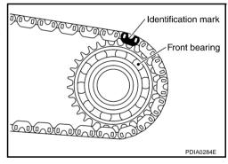
4. Install drive chain to mainshaft, and then install tap front drive shaft with plastic hammer. Press-fit rear bearing of front drive shaft to rear case.
