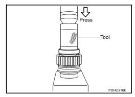
2. Install front drive shaft rear bearing, using the drift.
