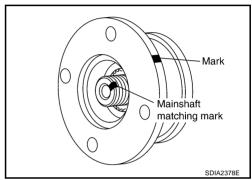
4. Remove the companion flange using a puller.
