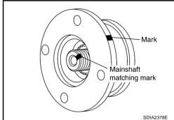
3. Using a flange wrench, install the self-lock nut of companion flange and tighten to the specified torque. Refer to  $\overline{\text{TF-45}}$ ,  $\underline{\text{"COMPONENTS"}}$ .
