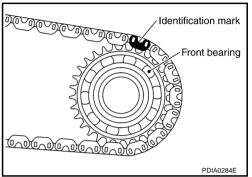
13. Install drive chain to mainshaft, and then install tap front drive shaft with plastic hammer. Press-fit rear bearing of front drive shaft to rear case.
