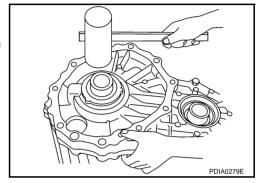
18. Tighten front case and rear case fixing bolts to the specified torque. Refer to <a href="TF-45">TF-45</a>, "COMPONENTS"</a>.
