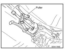
5. Remove the rear oil seal using the puller.
