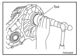
24. Install front oil seal until it is flush with end face of front case, using the drift.
