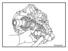
14. Remove oil gutter from rear case.
