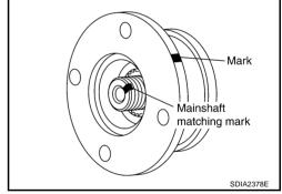
6. Remove companion flange, using a puller.
