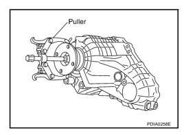
7. Remove rear oil seal from rear case, using the puller.
