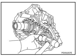
14. Install mainshaft bearing to front case, using the drift.
