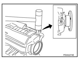
3. Install rear bearing to rear case, using the drift.
