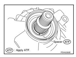
20. Install rear oil seal to rear case, using the drifts.
