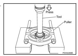
4. Remove front drive shaft rear bearing, using the drift and puller.
