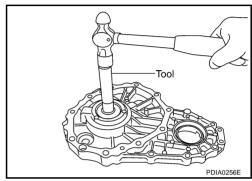
13. Remove drive chain and front drive shaft while tapping front drive shaft with plastic hammer.
