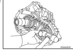
3. Remove front drive shaft front bearing, using the drift and puller.
