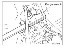
3. Put matching mark on the end of the mainshaft. The mark should be in line with the mark on the companion flange.
